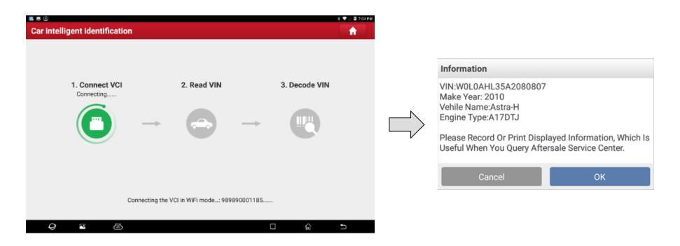
The vehicle model, manufacture year can be found automatically through the VIN number. This function is more convenient than manual selection.
